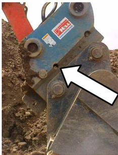
A quick hitch on an excavator enables fitting of different attachments to the dipper arm of a machine. It is a latching device which improves efficiency & productivity by aiding interchangeability of common attachments.
