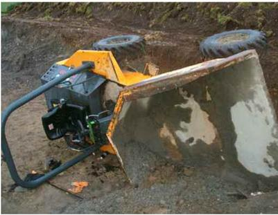
Roll Over Protection System or ROPS are designed and fitted to machinery which on overturning would reduce the possibility of an operator from being crushed, provided the operator was wearing a seat belt. The following points must be taken into account when operating plant with a Roll Over Protection System.
